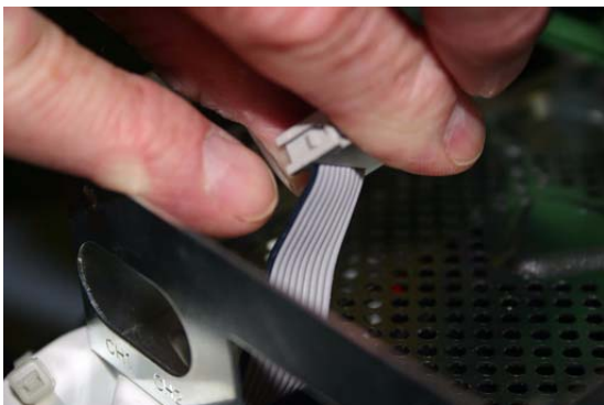
Figure 9 Pull the ribbon cable up
