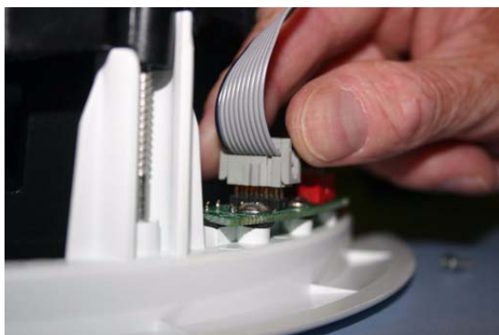
Figure 12 Press the ribbon connector back onto circuit card
