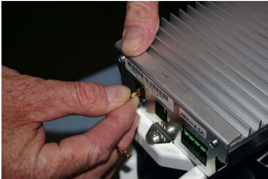
Figure 14 Attaching tweeter wires
