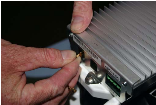
Figure 2 Removing tweeter wires
