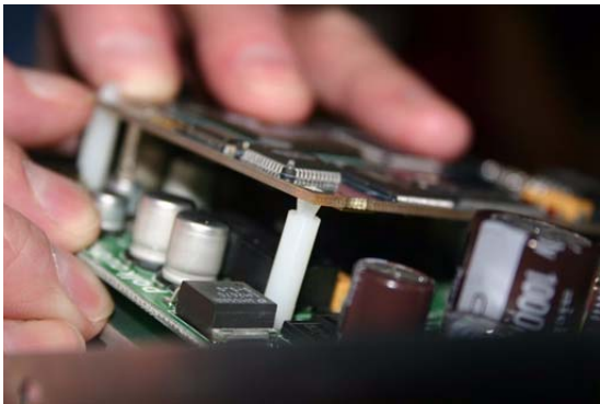
Figure 7 Pressing card onto standoff posts
