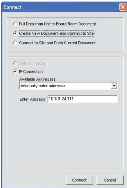
Console polls all units when a new site file is created, and automatically adds any new units on the expansion bus to the site.
