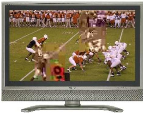
Packet Loss with a compressed signal being distributed over the network, causes blurry areas in the picture.
