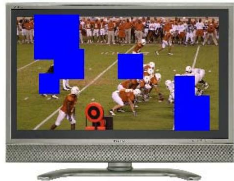
Packet Loss (with an uncompressed signal being distributed over the network), causes color blotches.
