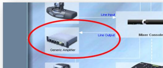
If you are using the Record Output for your external amplifier, drop the Generic Amplifier onto the icon for the Record Output and the icon will change appropriately.
