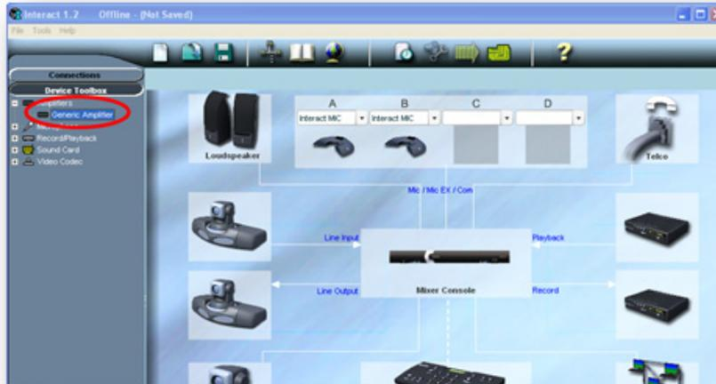
Open the Device Toolbox, open Amplifiers, and select the Generic Amplifier. With your mouse, grab the Generic amplifier icon, drag it and drop onto the correct output.
