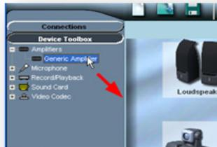
If you are using the Line Output for your external amplifier, drop the Generic Amplifier onto the icon for the Line Output.
