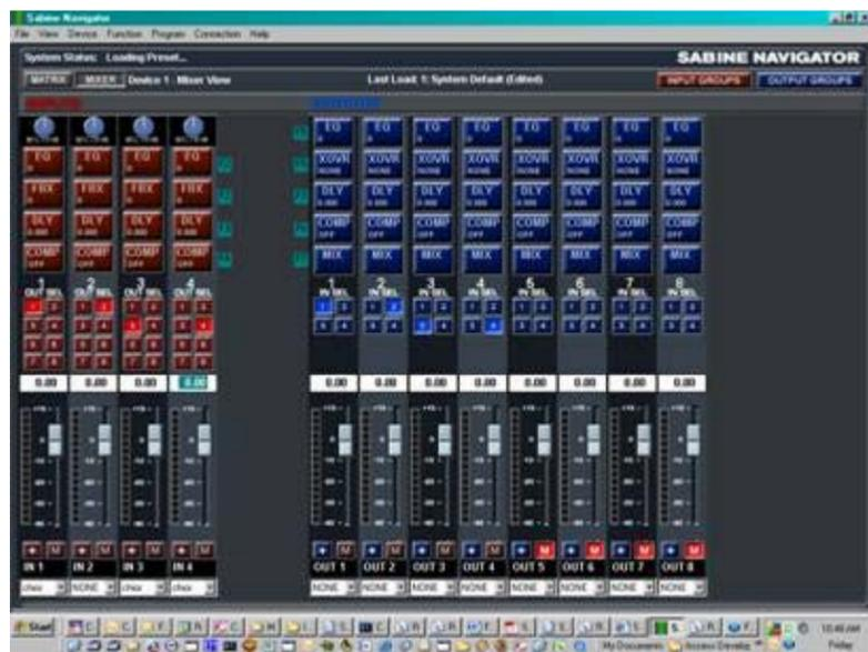
1. Set all the input and output sliders to 0 dB gain.
