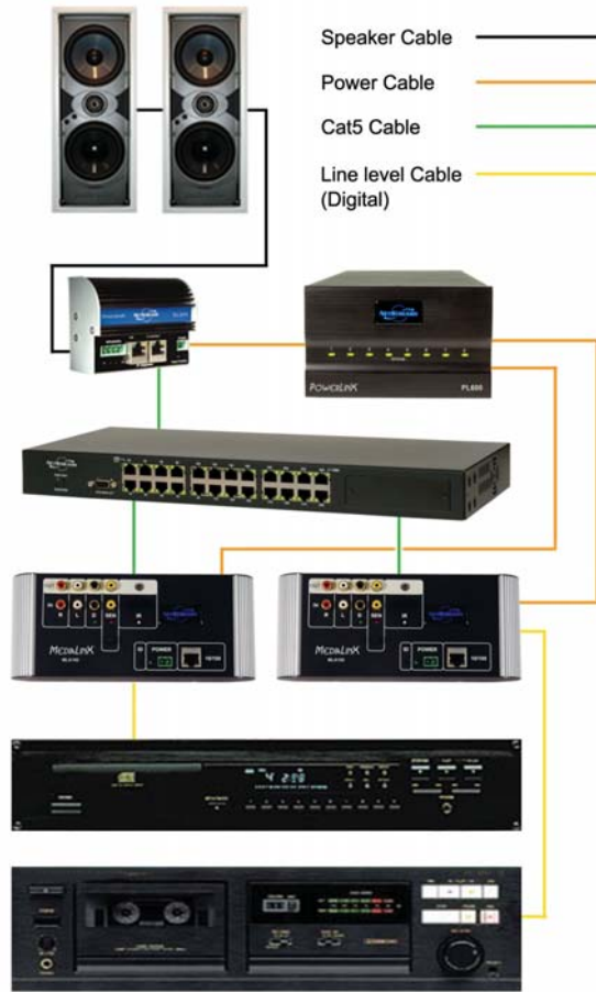
Figure 4: Pure Digital Signal all the way to the Speakers
