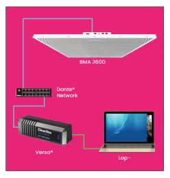
Connect the BMA 360D and Versa USB22D to a network using standard Cat 6 cables.
