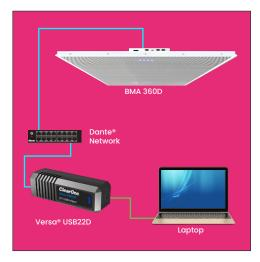
Versa USB22D enables any computer to be used with the ClearOne BMA 360D ceiling tile beamformer.
