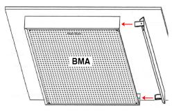
Warning! Surface mount kit must be independently supported by building structure according to all applicable national and local codes.
