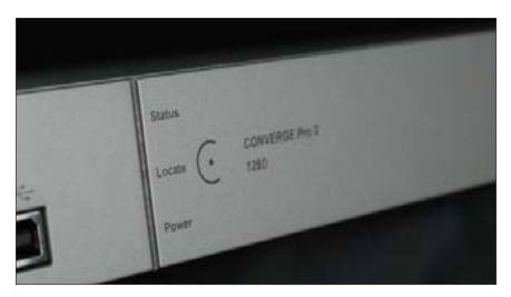
An advanced multi-channel microphone automixer with built-in support for Dante audio networking, and the latest audio DSP algorithms.
