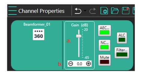
**Note:** Gain controls, Mute and Filtering options only apply to the SmartMix Dante Channel 13 output and do not affect the individuated Dante Beam output Channels 1-12.
