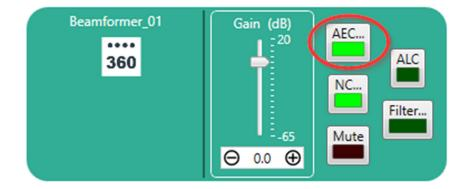
The AEC function provides full bandwidth (20Hz to 22kHz) echo filtering of the microphone signal. It uses a reference source (Dante input 5) which should include a mix of all far end participant receive audio that is being delivered to the room speakers.
