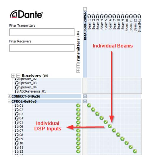
For simple room designs, utilize the SmartMix output 13 with integrated AEC, noise cancellation, filtering and zone mixing features. Utilizing the SmartMix microphone output and the built in amplifier channels, a complete system for cloud conferencing can easily be achieved. Below is a routing example using the Dante Virtual Soundcards (DVS) software on a PC for cloud conferencing. This example also utilizes the BMA 360D 4 channel amplifier for in room audio.
