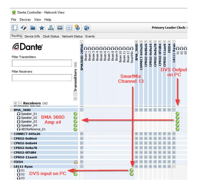
**Note:** That when using the SmartMix output, the AEC reference connection must also be used for proper Acoustic Echo Cancellation performance.
